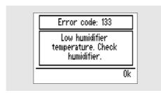
133: Low humidifier temperature. Check that the HA 01 humidifier is connected correctly (this error is shown after the treatment session). If the error remains, contact your care provider.
