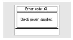
64: Low power. Check the power cables and the AC connection.
