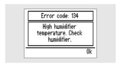
134: High humidifier temperature. Turn off the iSleep 20i. Disconnect the HA 01 humidifier and reconnect it. If the error remains, contact your
