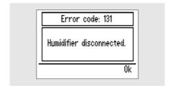
131: The HA 01 humidifier has been disconnected when the iSleep 20i was running. Always turn of the iSleep 20i before disconnecting the HA 01 humidifier.
