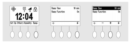
Use the 4 buttons under the display to navigate in the menu. Depending on the location in the menu, the buttons have different function and are called "soft buttons". The following icons are used:
