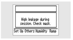
The leakage has been too high during the night for an accumulated time longer than 30 minutes. Check the mask fitting.
