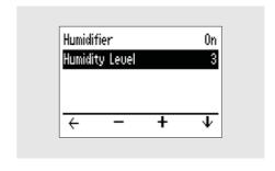
When the "Humidity" section is available in the menu, the HA 01 humidifier can be activated and deactivated by pressing and holding the "Humidity" soft button until the humidity symbol appears/disappears.
